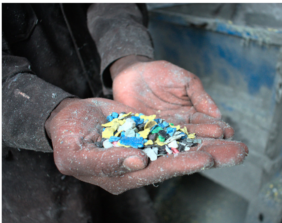
Crushed plastic, sand and color pigment are mixed together and fed into an extruder and heated to almost 400° C. The mixture is then placed into molds and compressed with a hydraulic press.
